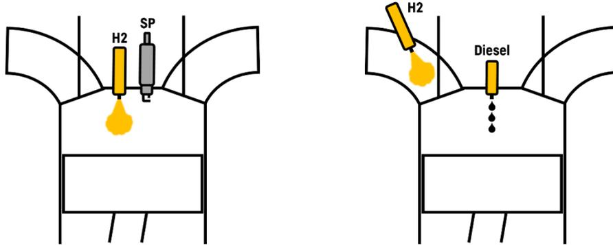
Figure 6: Engine configurations: DI : Direct injection and DF : Dual Fuel
