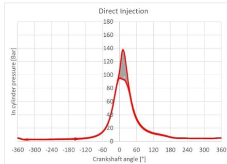
Figure 11: Cylinder pressure DI
