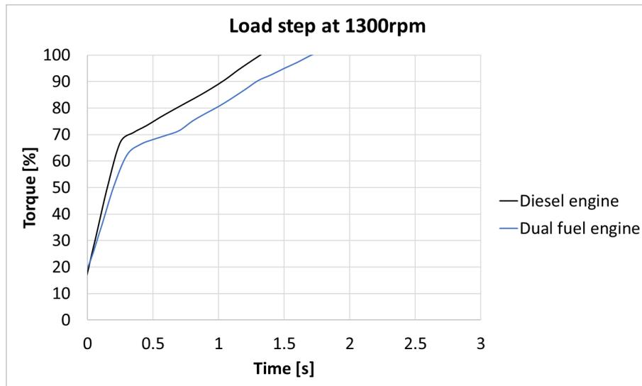
Figure 12: Engine dynamic for diesel and DF
