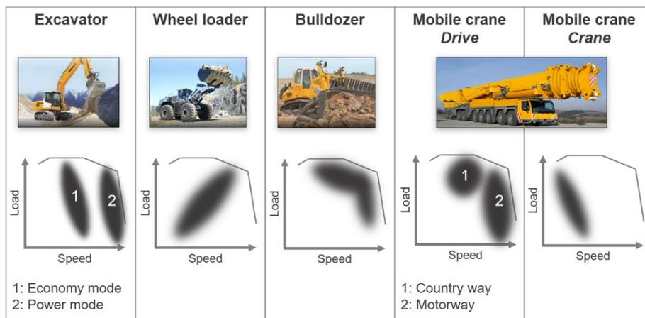
Figure 3: Operating cycles of Liebherr vehicles
