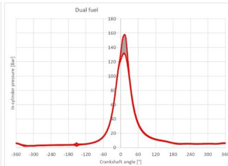
Figure 10: Cylinder pressure DF
