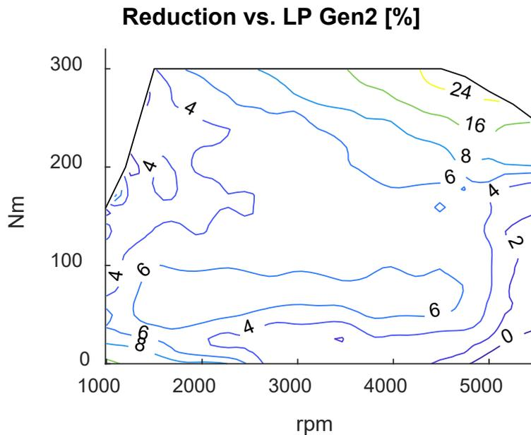
Fig. 9 BSFC reduction compared to VEP LP Gen 2.
