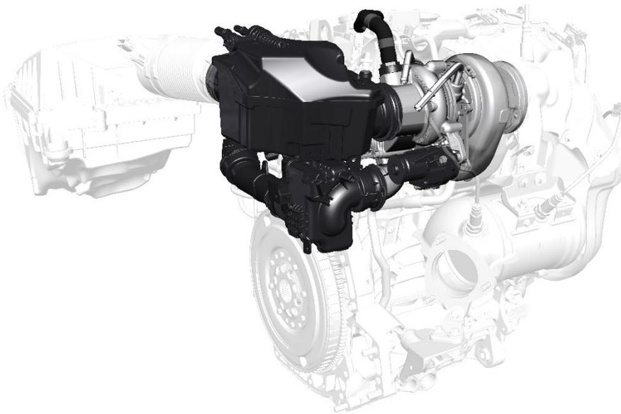
Fig. 3 Hot side of VEP LP with VTG Turbo and air routing and resonators.
