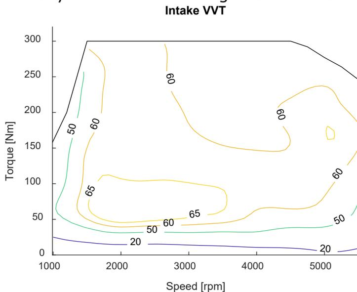
Fig. 5 Intake cam phaser position of VEP LP in steady state operation.
