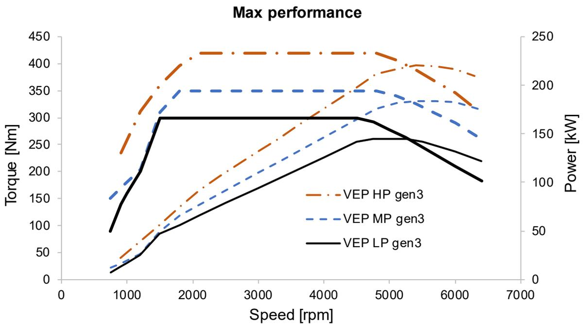
Fig. 1 Max torque and power of VEP Gen 3 LP, MP and HP.
