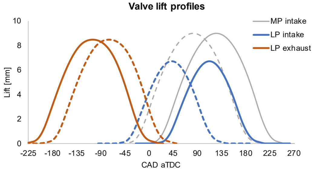
Fig. 4 Intake and exhaust valve lift profiles for MP and LP engine. Solid curves are cam phaser in base position and dotted curves its max position.
