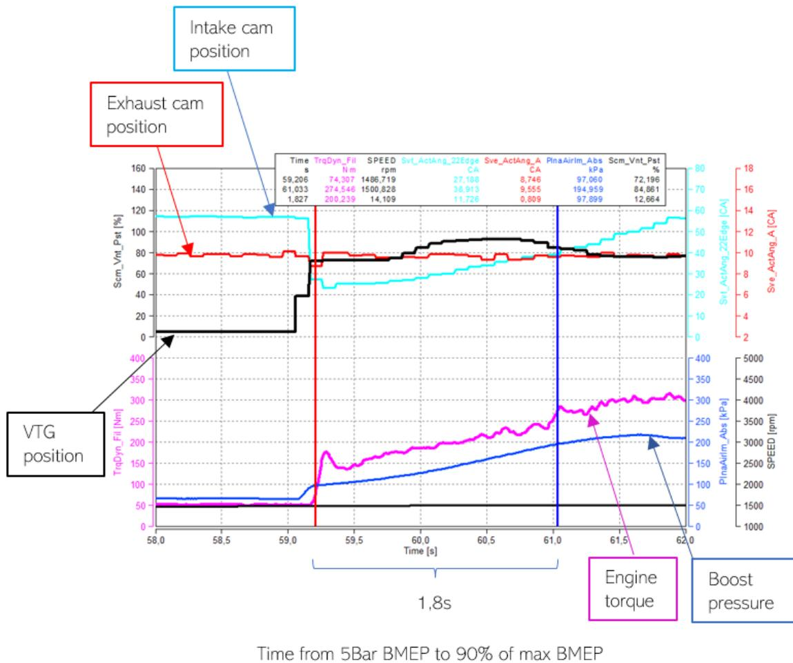
Fig. 10 TTT at 1500 rpm (only combustion engine without B-ISG).
