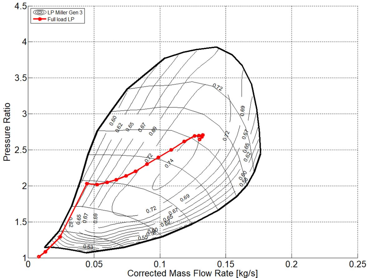
Fig. 13 VEP LP Gen 3 Compressor map including full load operation line.
