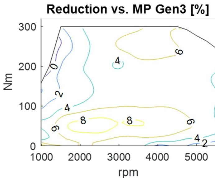
Fig. 8 BSFC reduction compared to VEP MP Gen 3.
