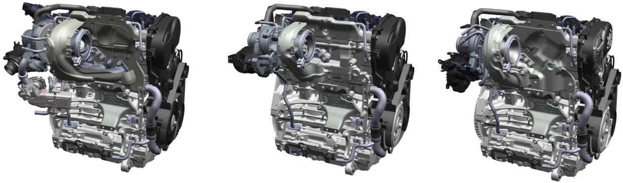
Fig. 2 VEP Gen3: HP (left), MP (middle) and LP (right).
